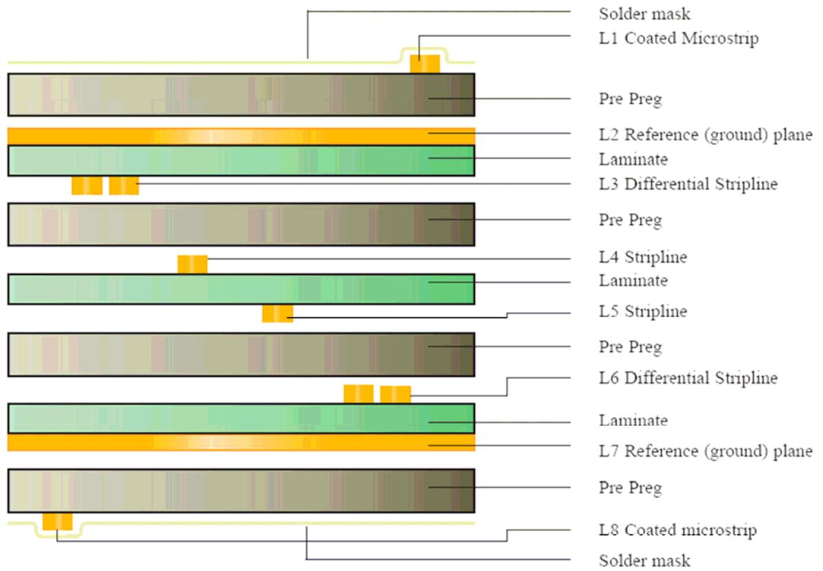
Exploded view of a test coupon 2
