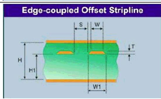
*This differential configuration has two traces that are separated by laminate and sandwiched between two planes. Although the diagram shows the traces offset, the manufacturing objective is to have the traces with no offset, i.e. one should be directly above the other. Typically, this configuration is difficult to fabricate.*
