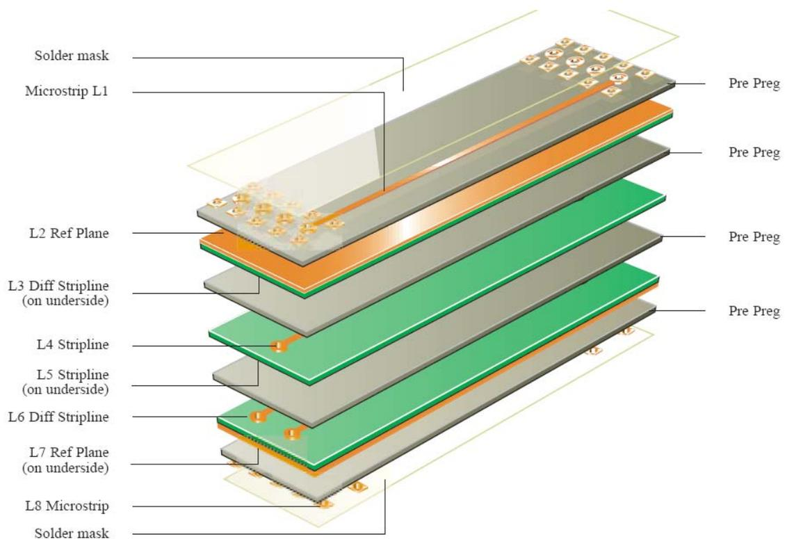
Exploded view of a test coupon 1
