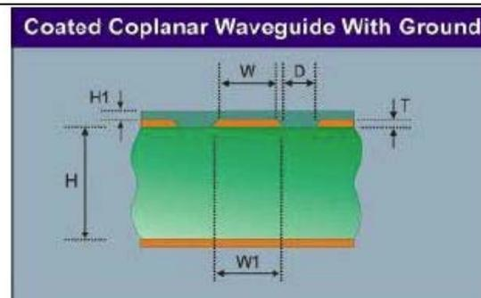
*This Coplanar Waveguide is similar to the above configuration except that there are planes on both sides of the laminate as well as a plane on the same layer as the controlled impedance trace.*
